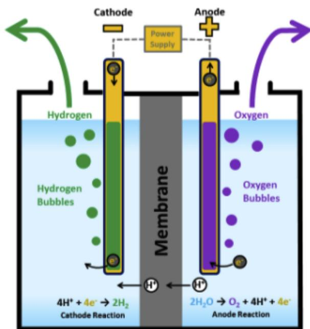
Fig. 1 – Electrolysis process in PEM [52].
